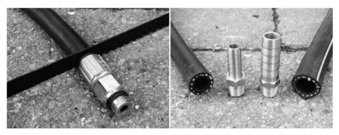
INSERT THE TAIL END INTO THE HOSE AND FASTEN A HOSE CLIP IN THE SAME WAY AS 7. (D).
