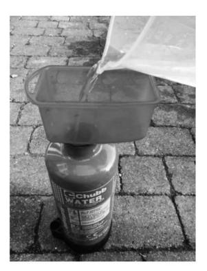
FIRST TRY WATER TO TEST YOUR MODIFICATIONS. THEN -FOR PAINT MIXTURES TRY 1 PART PAINT TO 1 PART WATER, OR IF ON A BUDGET THEN AT LEAST A RATIO OF 1:2. BE SURE TO MIX THEM TOGETHER. MATT EMULSION WORKS WELL AND IS MORE PERMANENT. POSTER PAINT IS CHEAPER AND ALSO WASHABLE.
