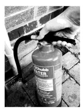
SOME WATER EXTINGUISHERS ALSO CONTAIN A FOAM ADDITIVE SO IT IS BEST TO DISCHARGE ALL WATER EXTINGUISHERS INTO A FOUL SEWER, NOT JUST FOAM ONES.
