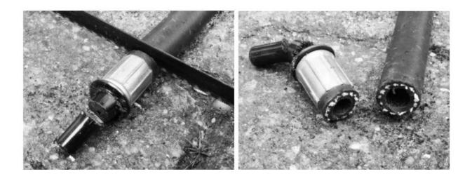
THE PROBLEM NOW IS THAT THE INSIDE OF THE HOSE WILL HAVE A LARGER INTERNAL DIAMETER THAN THE HOSE CONNECTOR, ESPECIALLY ON A JET SPRAY HOSE. WHETHER IT WILL STILL PRODUCE AN ACCEPTABLE JET DEPENDS ON HOW BIG THE DIFFERENCE IS – TEST IT. A BETTER OPTION IS TO MAKE A NEW NOZZLE (SEE NEXT SECTION).
